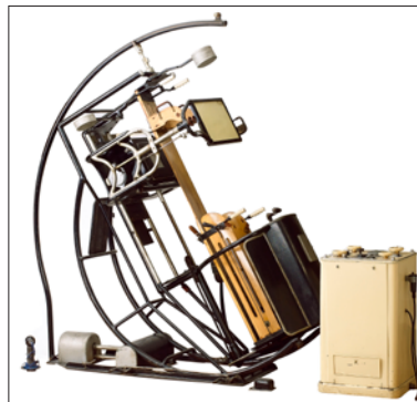
Pohl Omniskop X-ray apparatus ca. 1910, Germany metal, wood, glass, rubber, plastic 240 x 80 x 220cm Science Museum, London
