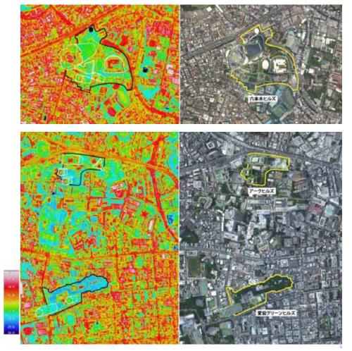
Pale blue parts in the thermograms above are areas where temperatures go up to around 30 , and red parts go over 40 . It shows the temperatures in areas with green space is 5 to 15 lower than the surface temperatures of areas paved with asphalt.
